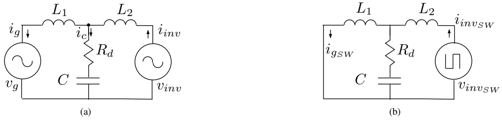
Fig. 4. (a) Per-phase equivalent circuit at fundamental frequency (b) Per-phase equivalent circuit at switching frequency
